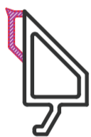
7201 (BLACK GASKET) GLAZING BEAD TO ACCOMMODATE 20/24 DOUBLE GLAZED UNIT
